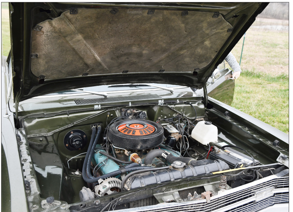
THE ‘69 Dart has a traditional 340 cubic inch engine with a 4 barrel carburetor. Jahnsen only plays old tunes on the push button radio in his Dart. The radio (right) is one of only two non-original items on the car. It’s an imitation with blue tooth capabilities.
