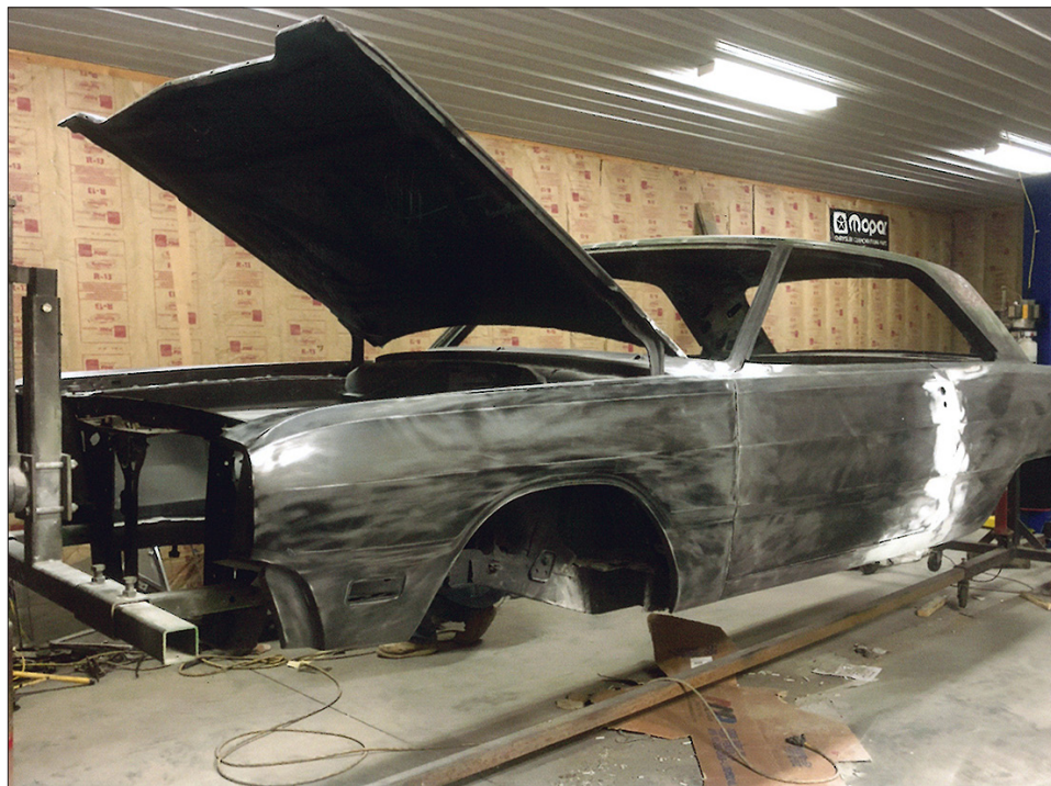
JAHNSEN ALSO refurbished this '67 Dodge Coronet R/T with a four-speed big block Hemi. Jahnsen uses a grinder on the back seat of the Dart Swinger(photo above right). The bare metal (below) is ready for the primer.
